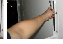
Begin to tighten <u>ALL</u> loose hardware on the remainder of the unit, being sure to align edges and bends of materials being tightened. This will square the unit to itself.
